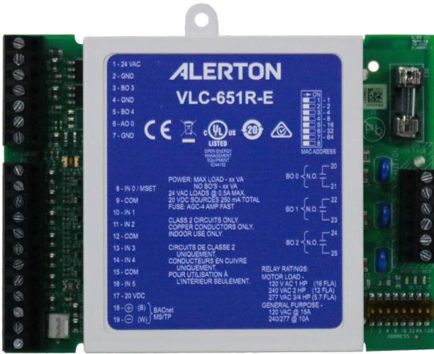
The Alerton VisualLogic® VLC-651R-E is a versatile, BACnet-compliant, fully programmable field controller, with three software-controlled high-current relays. The VLC-651R-E is well suited for unit ventilator and fan-coil applications, or any application that requires multi-speed fan or motor control. As a native BACnet controller, it integrates seamlessly with your BACnet system, communicating at up to 115 Kbps on a BACnet MS/TP LAN.
