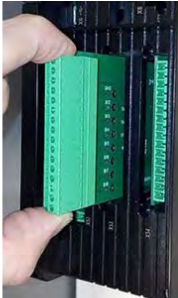
Figure 5-23. I/O module removal
