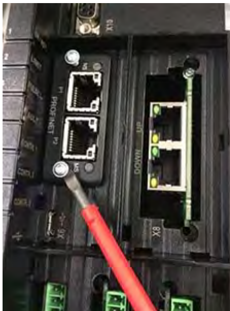
Figure 5-22. Anybus module removal
