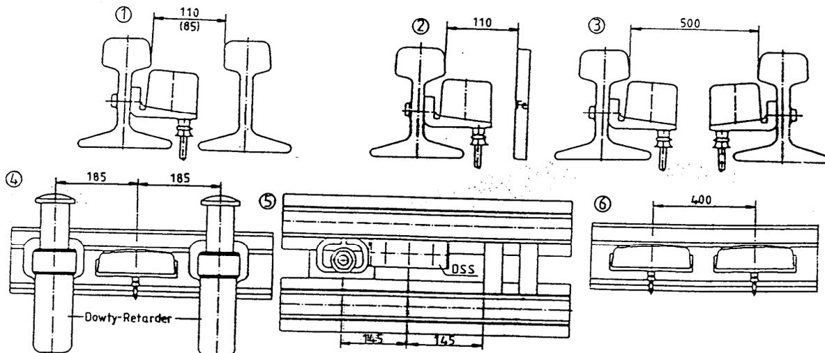
If the installation dimensions are arranged favorably, changes in the height of the wheel cannot destroy the switch.
