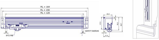
ML= Measuring length Dimensions in mm
